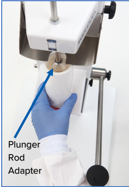
Plunger Rod Adapter used (250mL EMP Jar)
