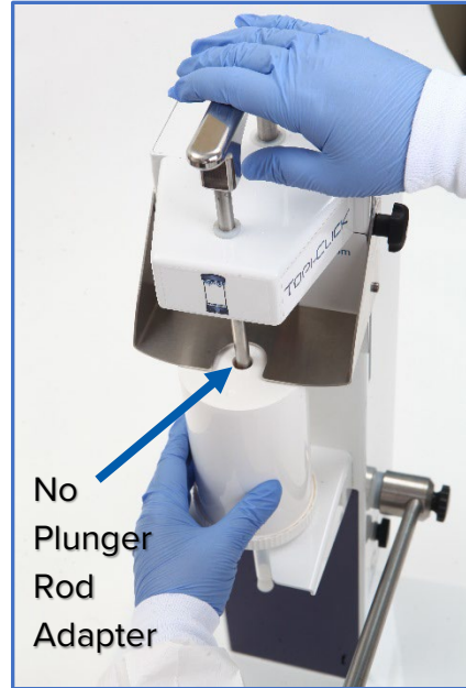
No Plunger Rod Adapter used with 500mL EMP Jar.
